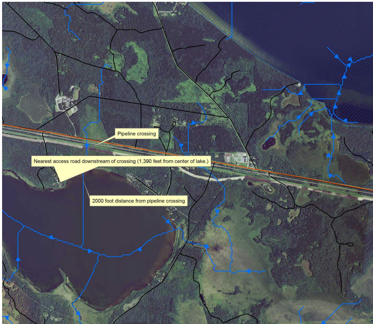
Figure E- With the wetland identifying layers turned off, one can see that there are no roads or upland areas from which to access potential leak sites at this crossing. There is a possible access point identified to the southwest of the pipeline crossing, but containment equipment would have to be strung across over 3,000 feet of wetland as it flows into the lake to contain all of a release as it flows to the south. (Scale 1:24,001)
