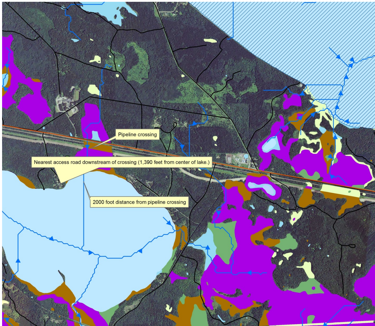
Figure D-With NWI wetland layer turned on, one can see wetland extending well beyond the 2,000 foot buffer at this crossing along the "Northern" route. The purple is bog, the green is forested wetland. In Figure E below the wetland layer is turned off so that accessibility to a potential leak here can be determined. (Scale 1:24,001)
