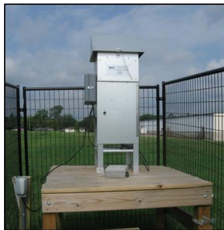
High-volume TSP Sampler
