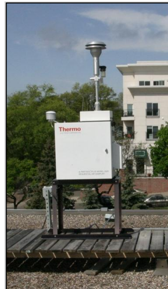
Low-volume PM 2.5 filter monitor
