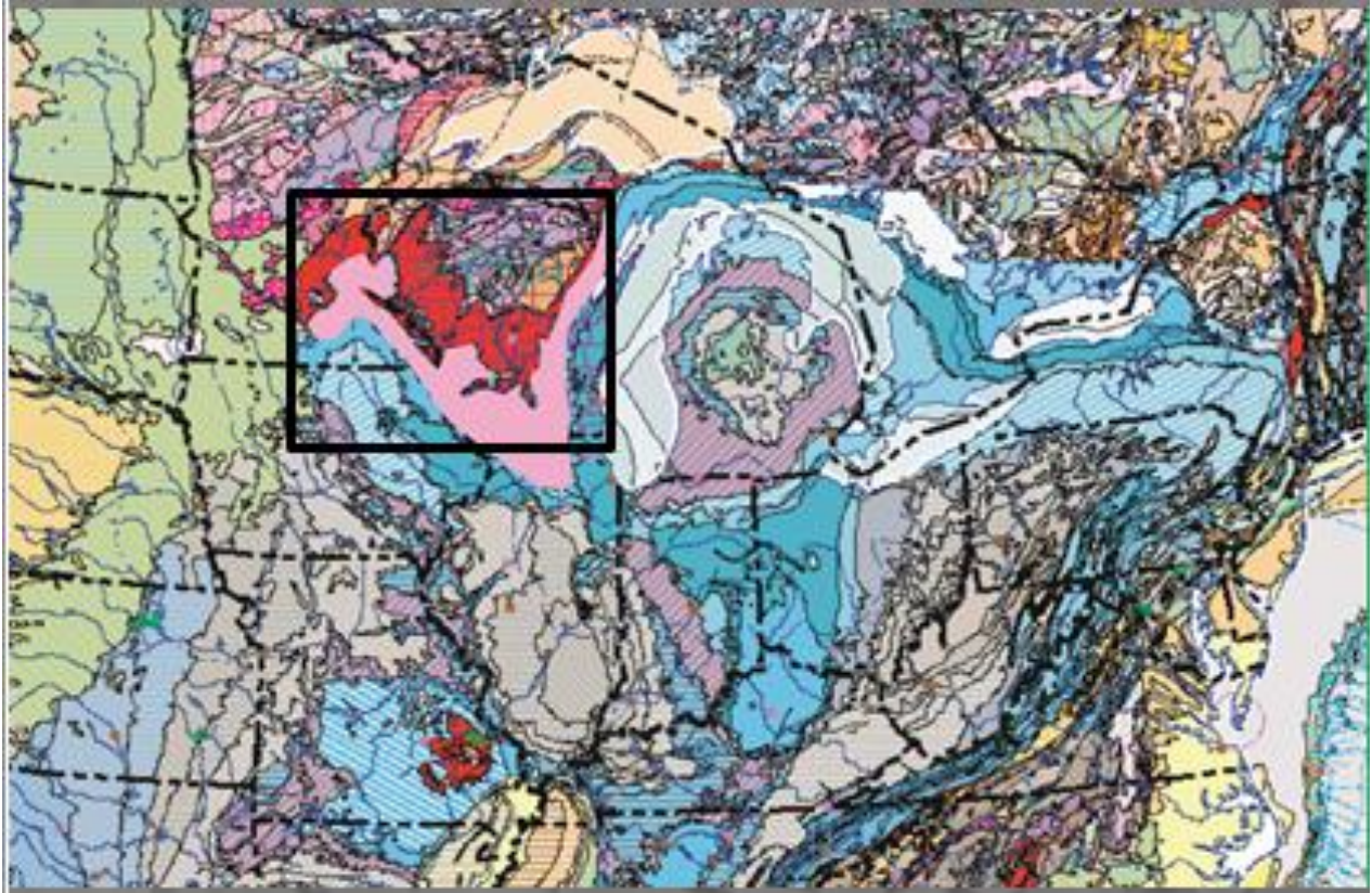
Figure 4. First encountered bedrock. Silica sand deposits are displayed in red and solid pink. Source: Runkel, 2012.
