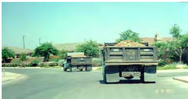
Figure 12. Untarped and overloaded hauling vehicles.
